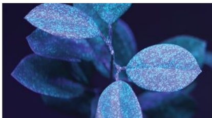
Spray Pattern from 3D Nozzle
