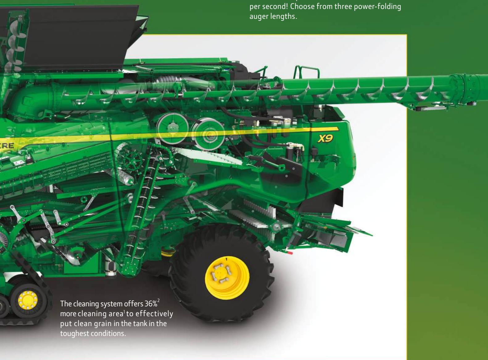
The cleaning system offers 36%<sup>2</sup> more cleaning area<sup>1</sup> to effectively put clean grain in the tank in the toughest conditions.
